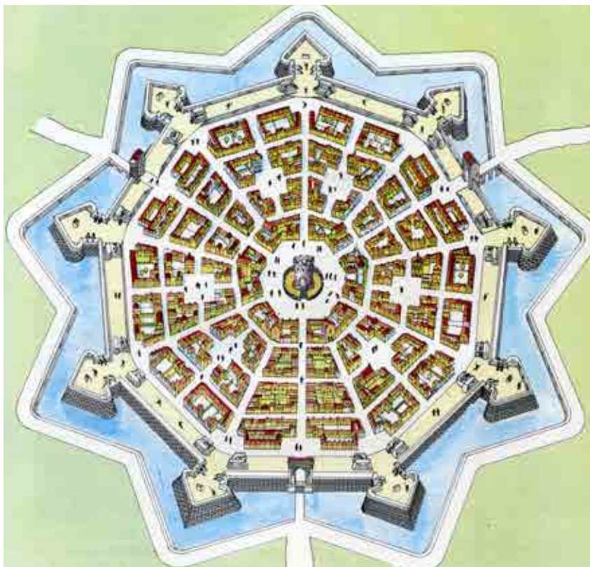
Palmanova, plan taken from an old print. This is a fortress town known also from its rather unusual plan as "the star-shaped town" ( la Città Stellata ). It was, in fact, founded in 1593 as a defense post on the frontiers towards Austria and its shape is perfectly symmetrical with nine points and a spacious square from which six streets radiate outwards. From Lugani, V. (ed.), Friuli Venezia Giulia , Aristeia, Milano, 1978.
